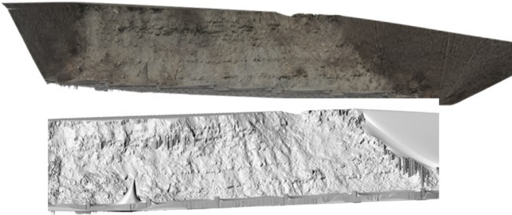
Figure 5. Photographs mosaic and hillshade representation of the digital elevation model generated from mobile SFM photogrammetry, at the Cincinnati site.
