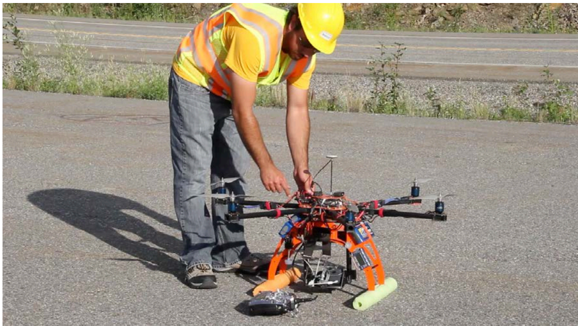
Figure 3. Hexacopter UAV used for SFM photogrammetry in the project.
