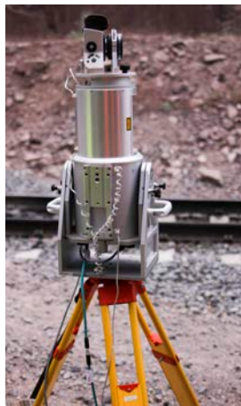
Figure 2. Riegl LMS-Z210ii instrument used to collect terrestrial LiDAR points at the field site in Nevada.
