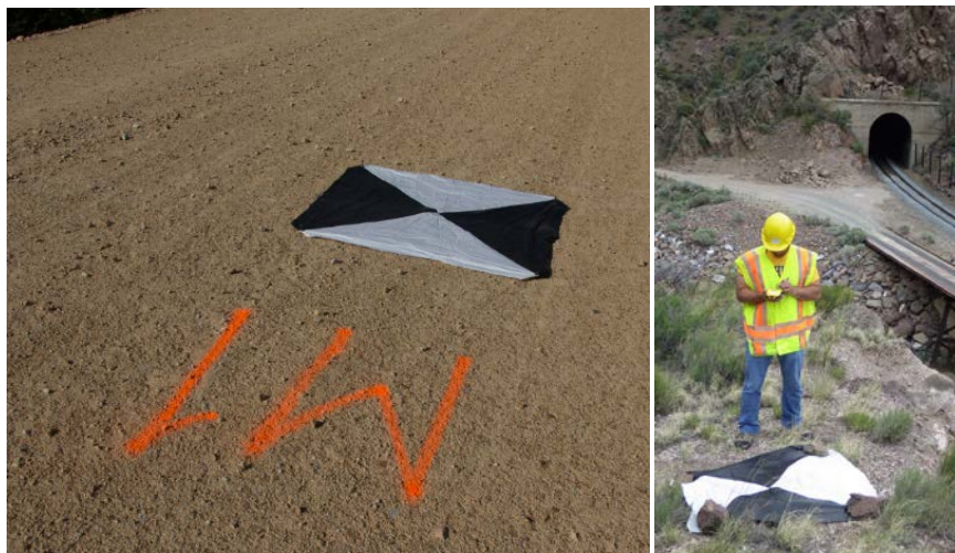
Figure 4. Plastic sheet field target for the ground control point. Left: target displayed on a road at the Alaska test site. Right: target displayed on a slope at the Nevada site.
